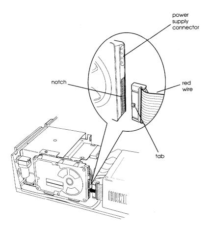
4. Make sure the holes in the cable connector fit over all the pins in the hard disk drive connector; then push in the connector.
